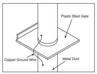
**Figure 15.** Ground jumper wire when using plastic blast gates or elbows and metal duct.
